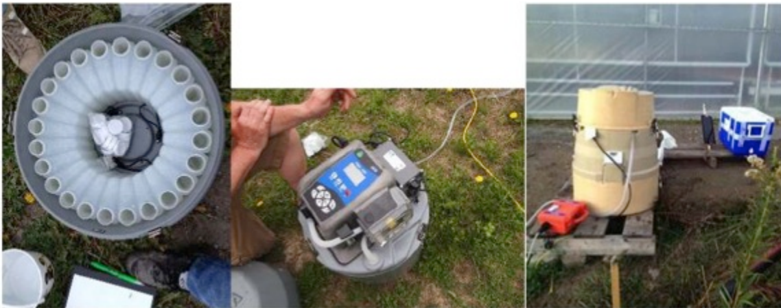
Figure 1 – Autosamplers used in the research study, showing interior sample collection basket, the control panel, and the setup at the greenhouse.
