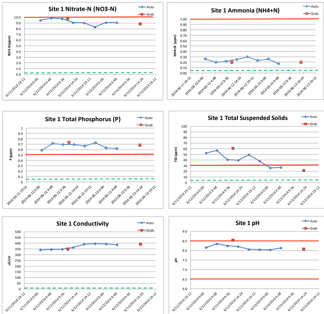
Figure 8 – Key parameters of Site 1 overflows over time, comparing grab samples with samples obtained with an autosampler. MOECC targets are marked in red lines (—) and analytical detection limits are marked in green hatched lines (-----)
