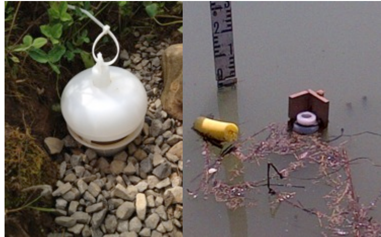
Figure 2 – Nalgene first flush (ping-pong) samplers used in the research study, placed in a swale that lead to one of the ponds, and in a pond mounted on a post.
