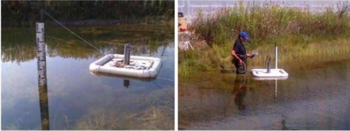
Figure 3 – Sensor and staff gauge setup in the ponds, where the sonde and water level meter are mounted in a floating ‘mat’. Sometimes getting the setup complete involved getting right in!
